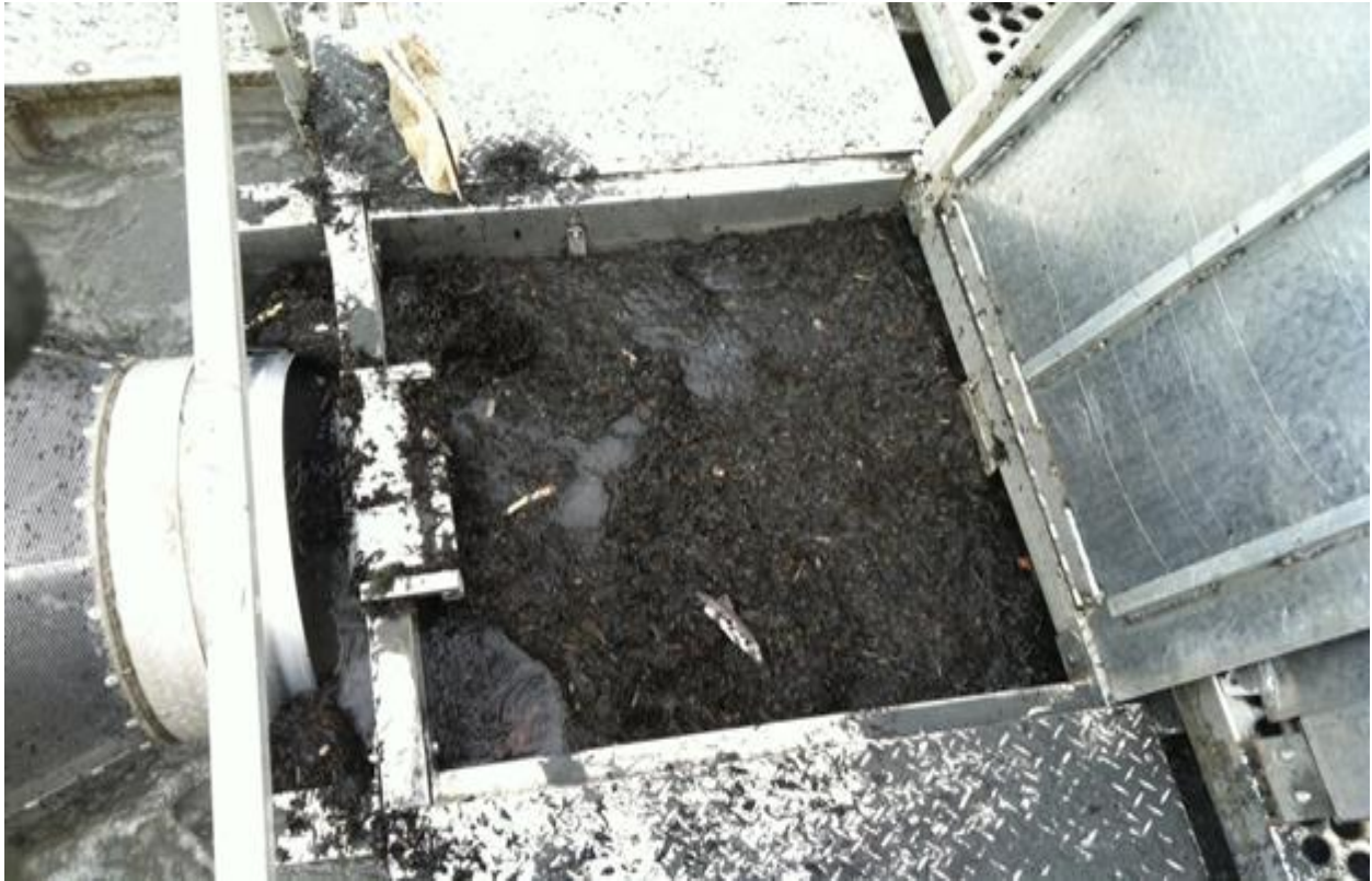
Figure 6. Mainstem Elwha River smolt trap filled with sediment and woody debris, spring 2013.
