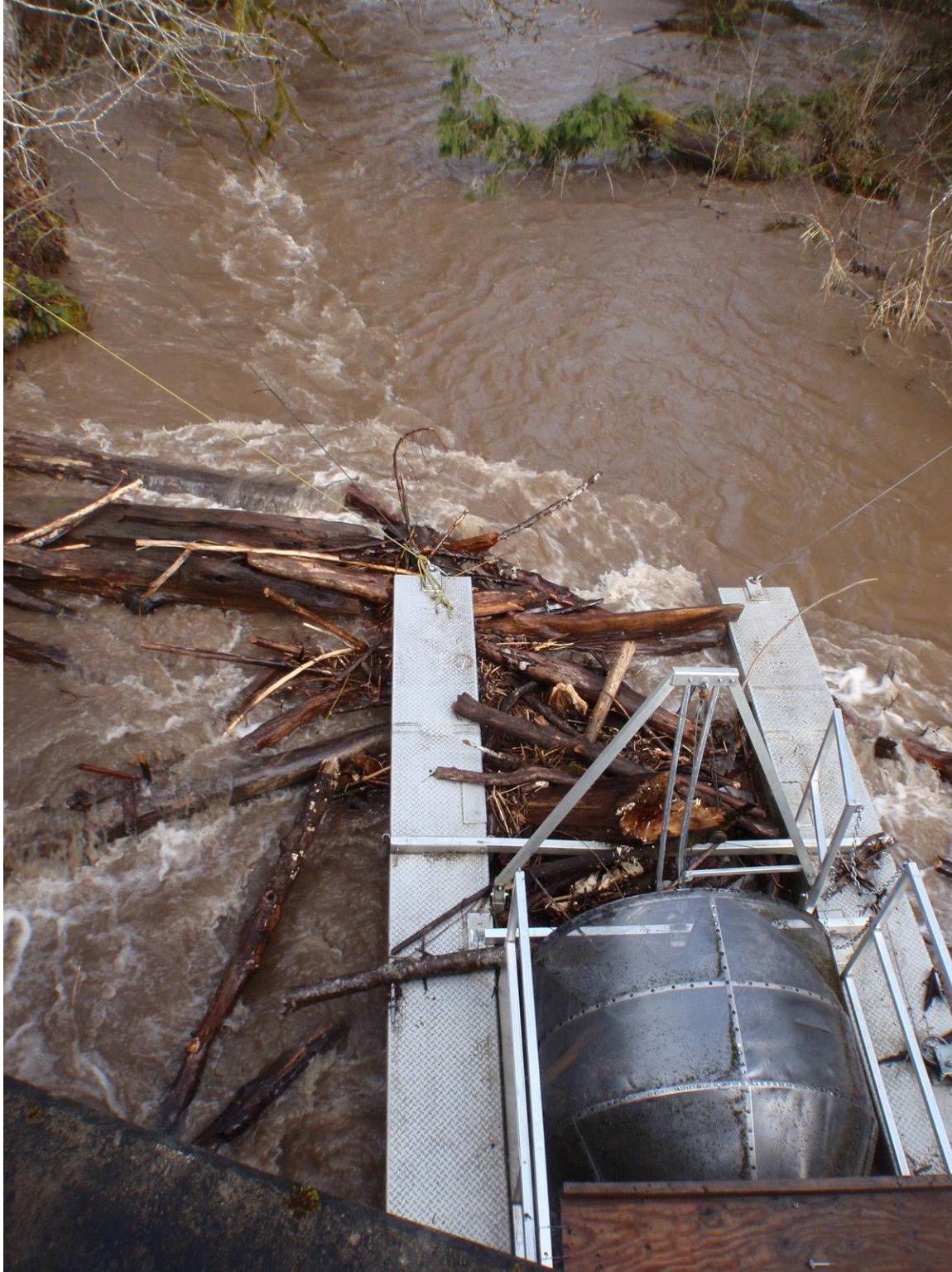
Figure 8. Woody debris entrained into Little River rotary screw trap, February 2014.
