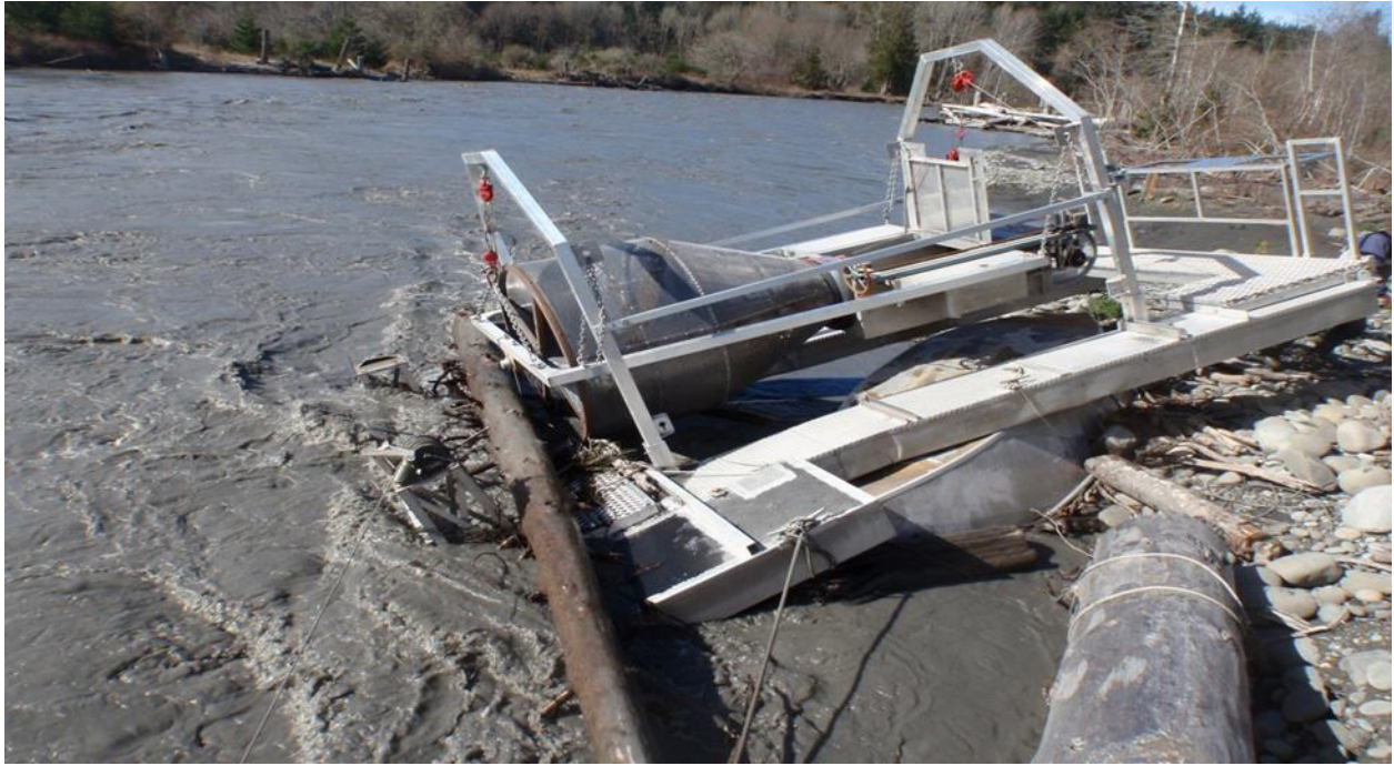
Figure 7. Mainstem Elwha River screw trap depicting damage from impact with fluvial transported wood, spring 2014.
